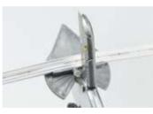
Use professional scissors to cut vertically at the cutting mark
