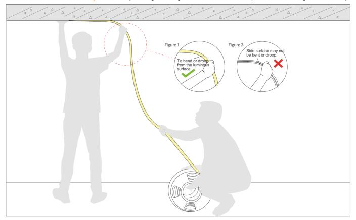
Installation Precautions - Top Mounted (If the length of the light is more than 2 meters, two persons must work together to install it.)
