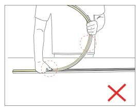
Do not press the led strip with a single finger, it is easy to damage the internal parts of the led strip.
