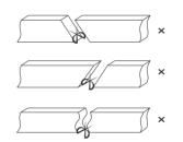
Please don't be feel free to cut and cut into an oblique angle or cambered section.
