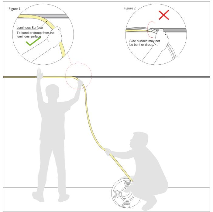
Installation Precautions - Side Mounted (If the length of the light is more than 5 meters, two persons must work together to install it.)
