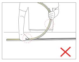
Do not press the led strip with a single finger, it is easy to damage the internal parts of the led strip. The bent arc of the led strip should not be too large during installation.
