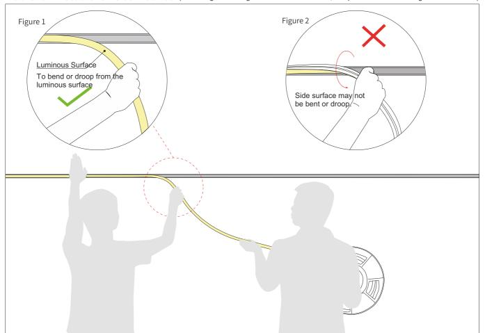
Installation Precautions - Side Mounted (If the length of the light is more than 2 meters, two persons must work together to install it.)
