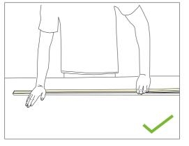
Please press the led strip with your palm to slowly insert the led strip into the groove, and gently straighten the led strip a bove the groove with your right hand.
